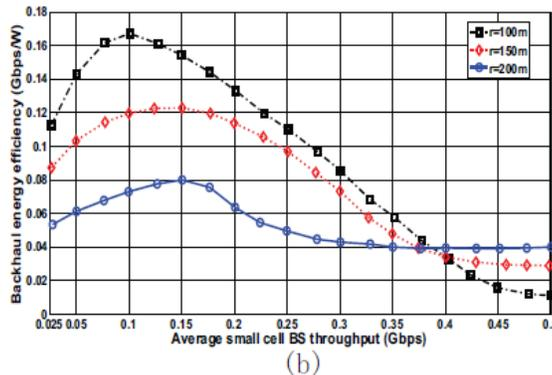
**Fig. 5.** Energy efficiency of ultra-dense cellular networks (b) backhaul energy efficiency vs average small cell BS throughput.
