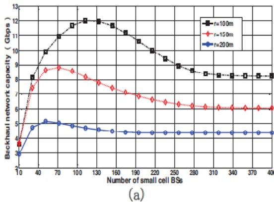
Fig. 2. Backhaul network capacity of ultra-dense cellular networks: (a) the backhaul network capacity vs the number of small cell BSs
