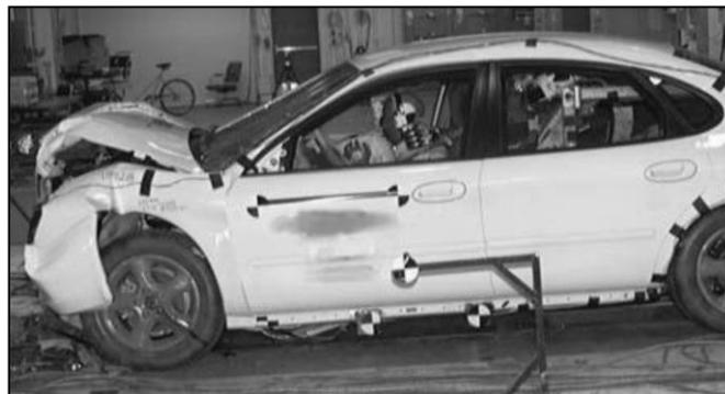
**Figure 1.** Mid-sized vehicle crash against a full rigid barrier
